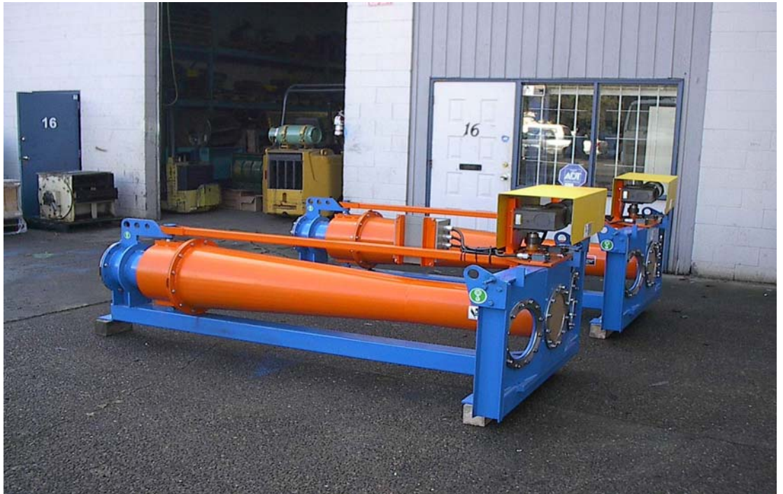
FIGURE 3.7 Two 10 ¾" A9 diverter valves 3 way ports.
